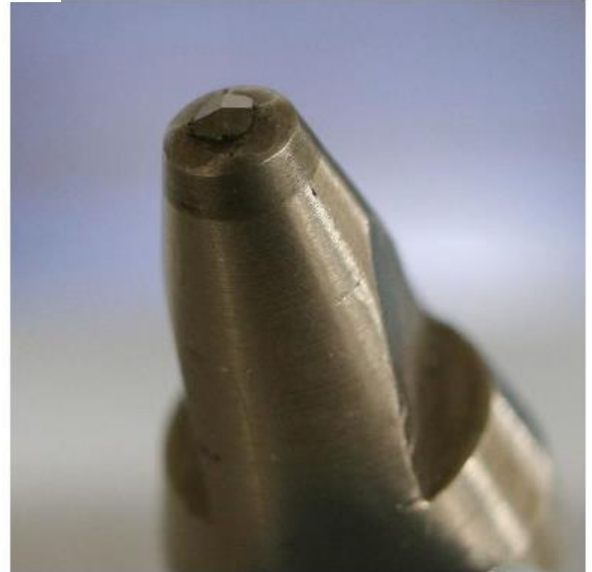
Vickers diamond indenter: the mount
