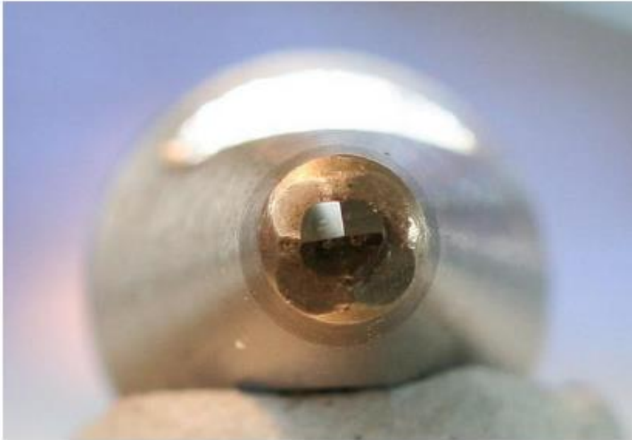
Vickers diamond indenter: the end
